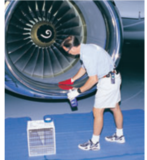
A Boeing Service Letter identifies XZilon as a temporary method of corrosion protection for the BBJ engine inlet.
